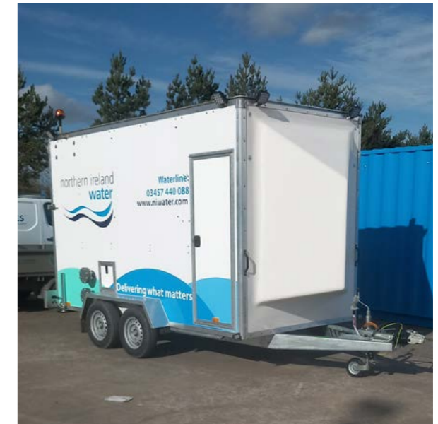
NI Water's second mobile booster trailer.
